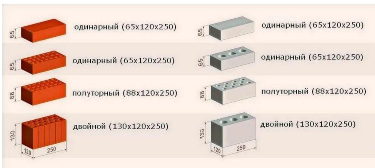
Fig. 16 - Standard brick dimensions according to GOST 530-2012.
