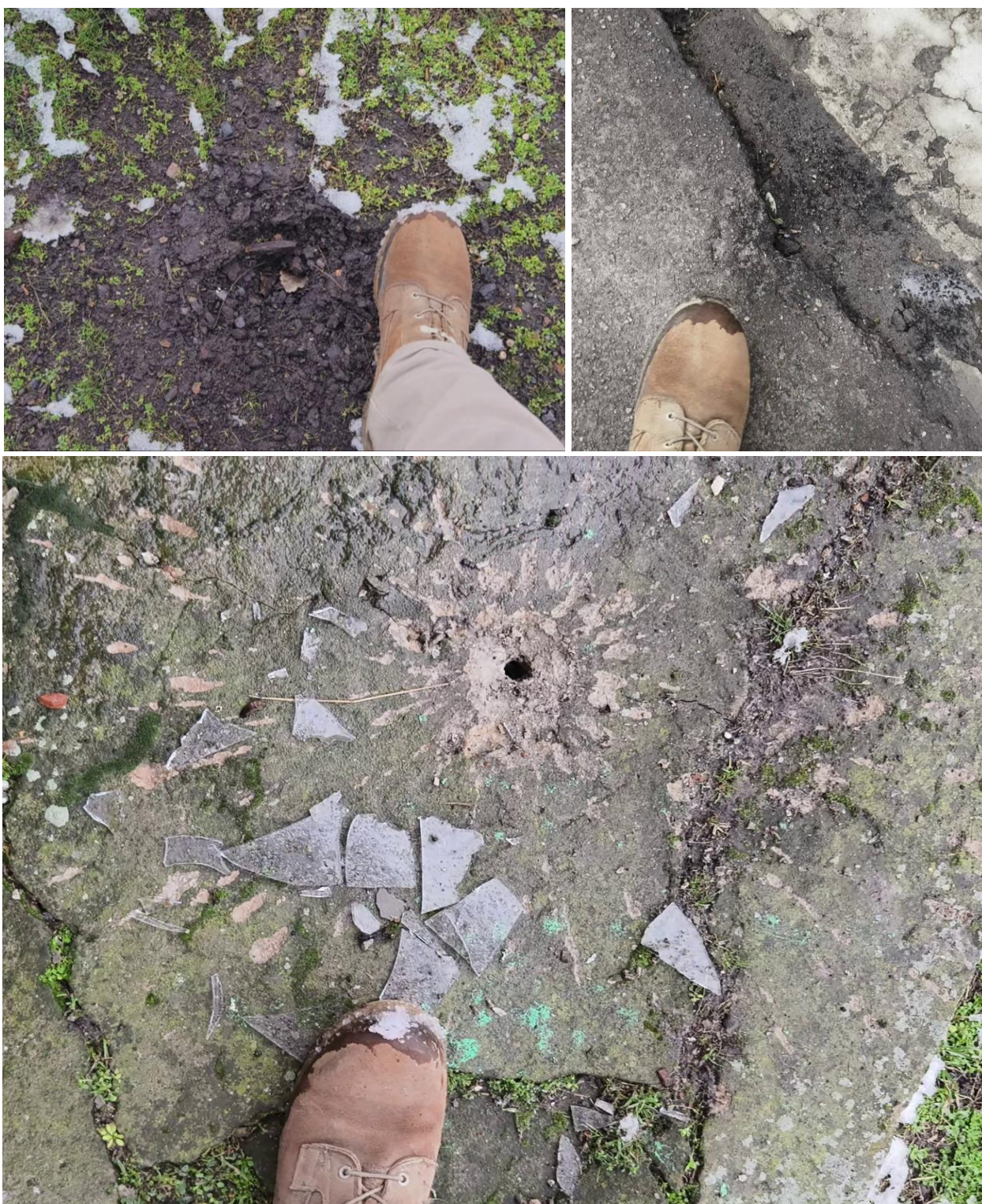
Fig. 10 - CSM explosion craters with an object of known dimensions in the frame: top left - in the courtyard of the Bekhtery school; top right - near the general merchandise store; bottom - on the bell cast surface near the wall of the Bekhtery school building.
