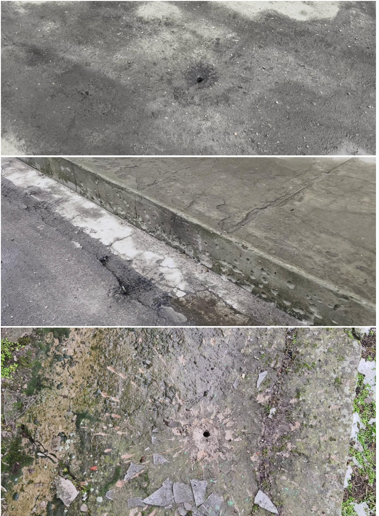
Fig. 12 - Examples of craters from KSB detonation on the solid surfaces.
