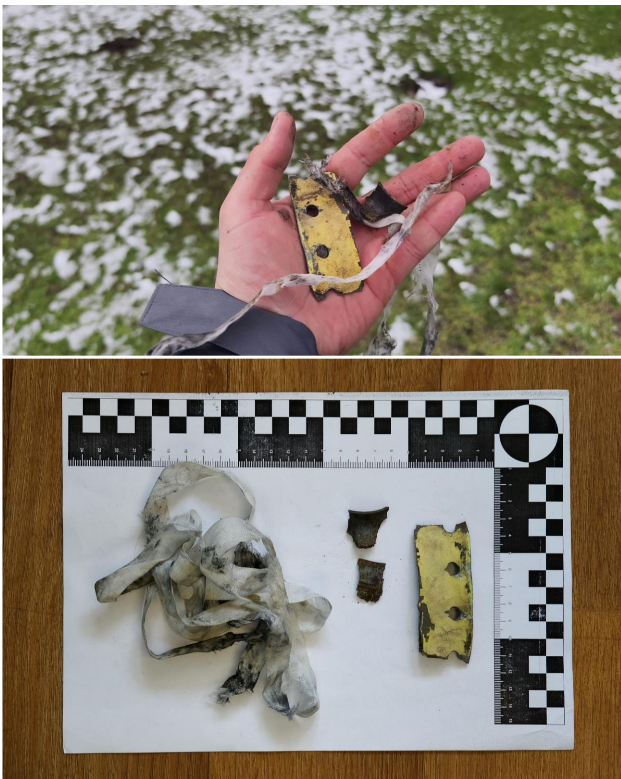
Fig. 20 - The remains of the projectile that we found during the inspection: on the right - CSM stabilizer belts; in the center - the CSM casing debris; on the right - the rocket casing debris.
