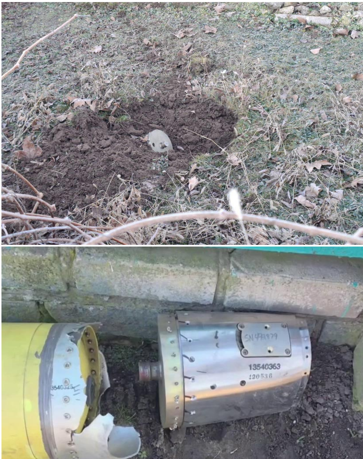
Fig. 14 - Guidance and control unit of a rocket projectile: top — sunk as a result of falling into the ground in the territory of a school in the village of Bekhtery; bottom — extracted by sappers.
