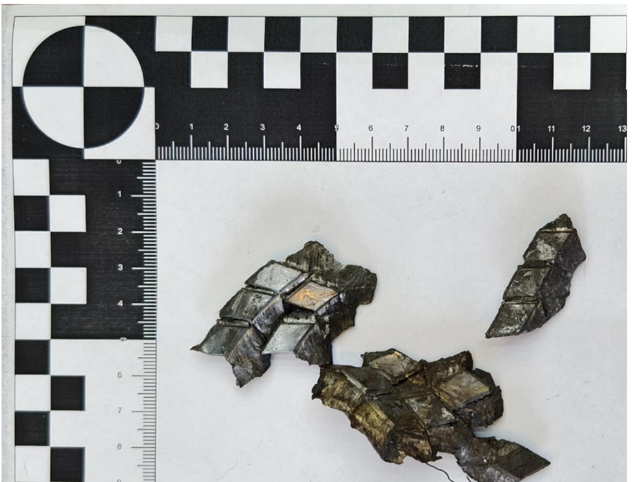
Fig. 8 - Fragments of the fragmentation jacket of a rocket projectile found at the sites of shell hits 4 and 6.
