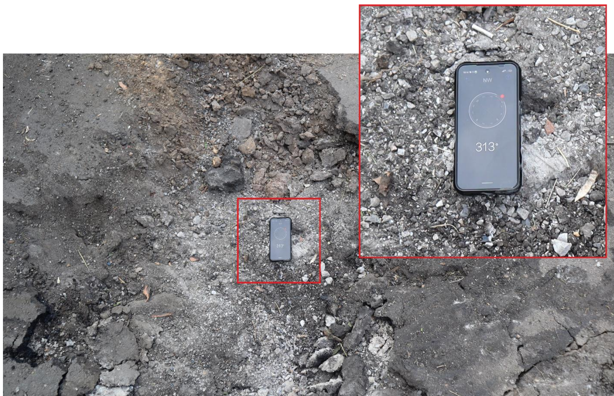
Fig. 13 – Determination of the shelling direction in the case of shell hit 1.
