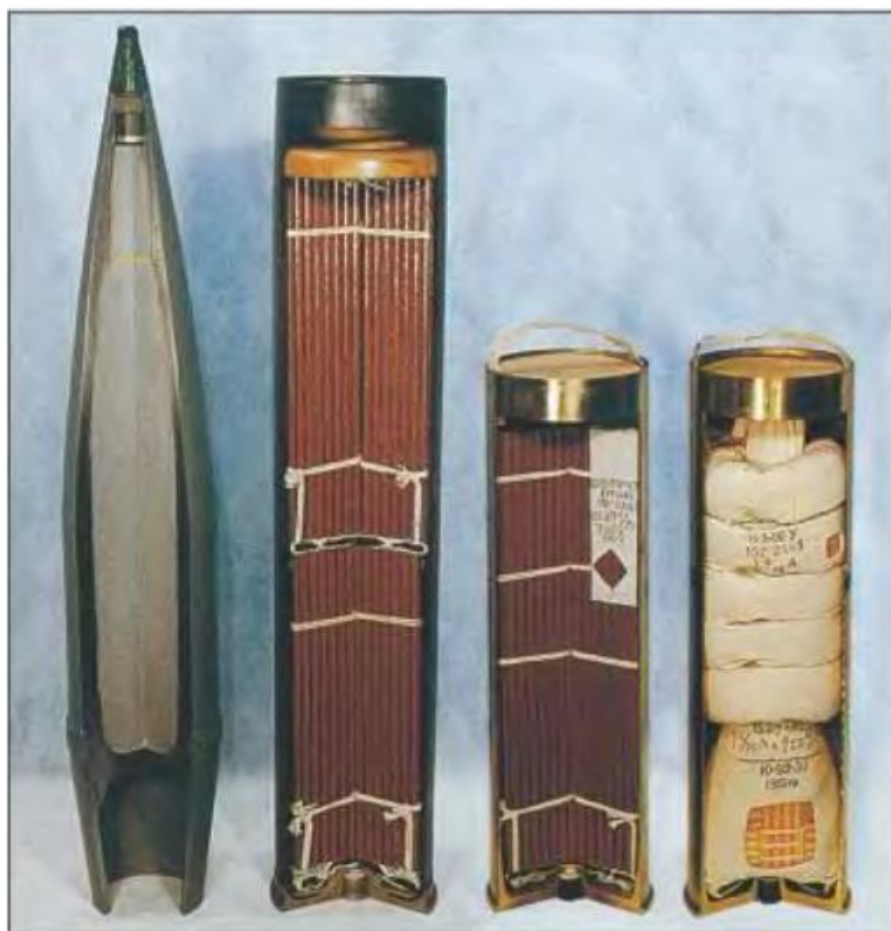
Fig. 9 – The ZOF45 projectile and various options of charges for it.
