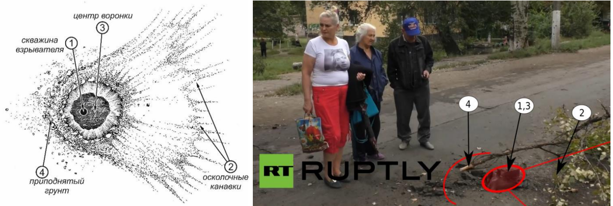
Fig. 27 - Scheme of a crater from a projectile hit at a large striking angle to the surface (left) and a real crater from a projectile hitting the road pavement opposite the north-east corner of the residential building at 11, Gvardeisky quarter (right) 30 .
