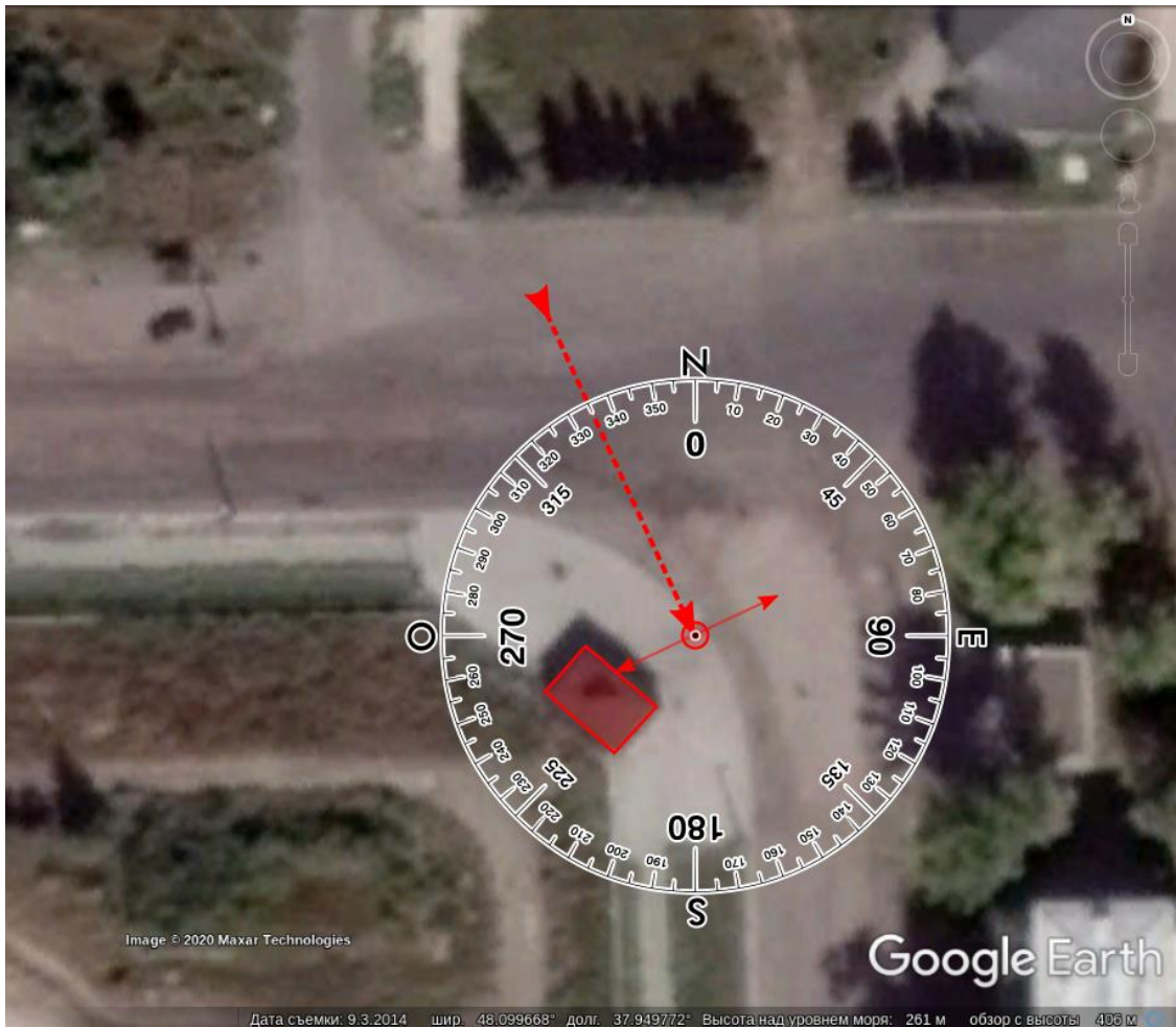
Fig. 29 – Scheme of fire direction determination using satellite imagery.
