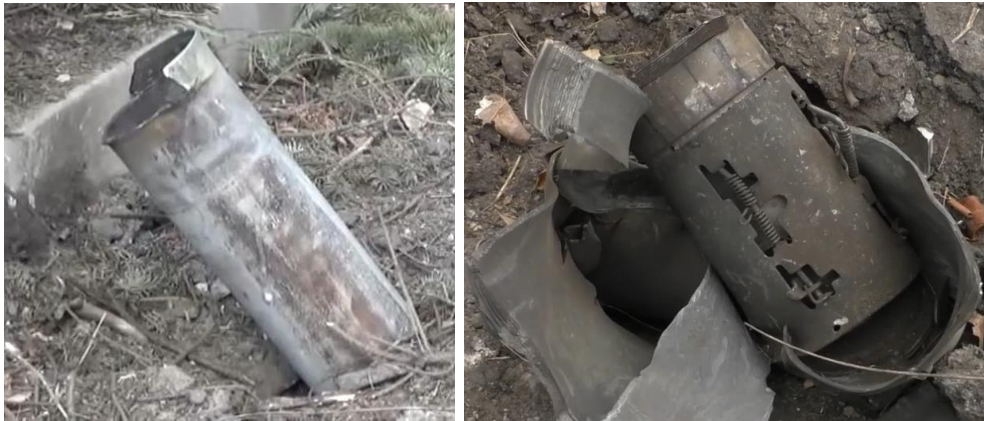
Fig. 12 – The remnants of the rocket part of the 9K51 Grad MLRS shell 14 .
