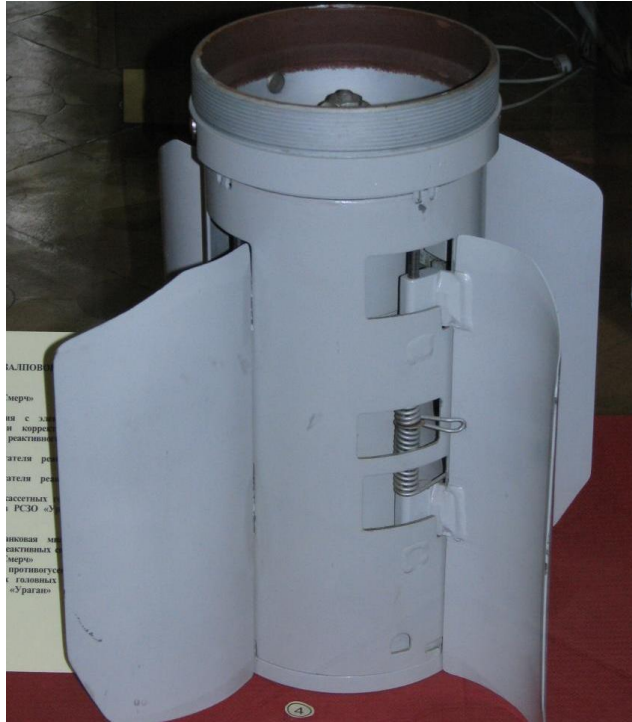
Fig. 15 – A dummy stabilizer control unit for the Uragan MLRS projectile 19
