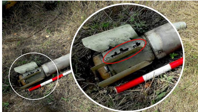
Fig. 17 – The remains of the 9K51 Grad MLRS projectile found near Krasnogorovka on 28.08.2016. 21
