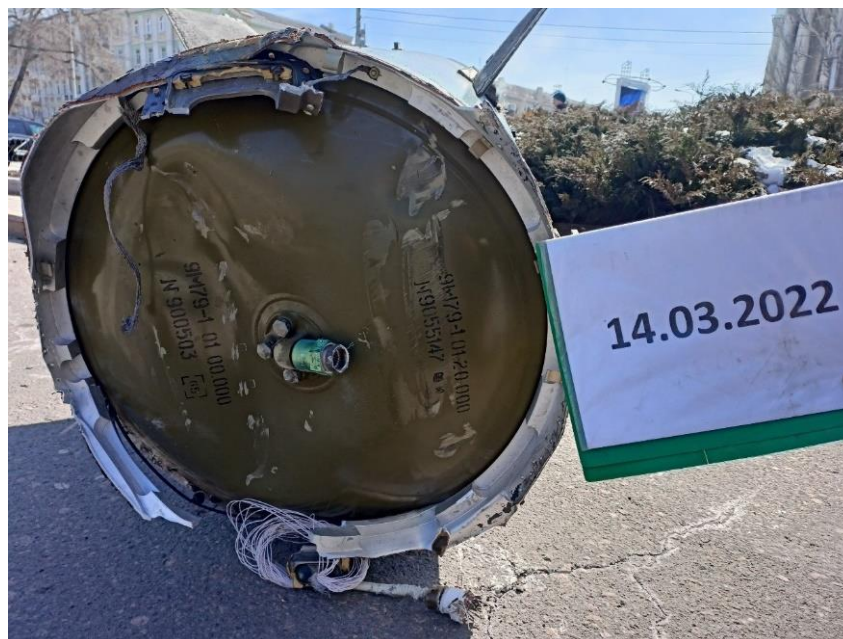
Fig. 16 – Marking on the end of the propulsion system of the Tochka-U missile, which fell at the intersection of Shevchenko Blvd and Artioma Str 48 .
