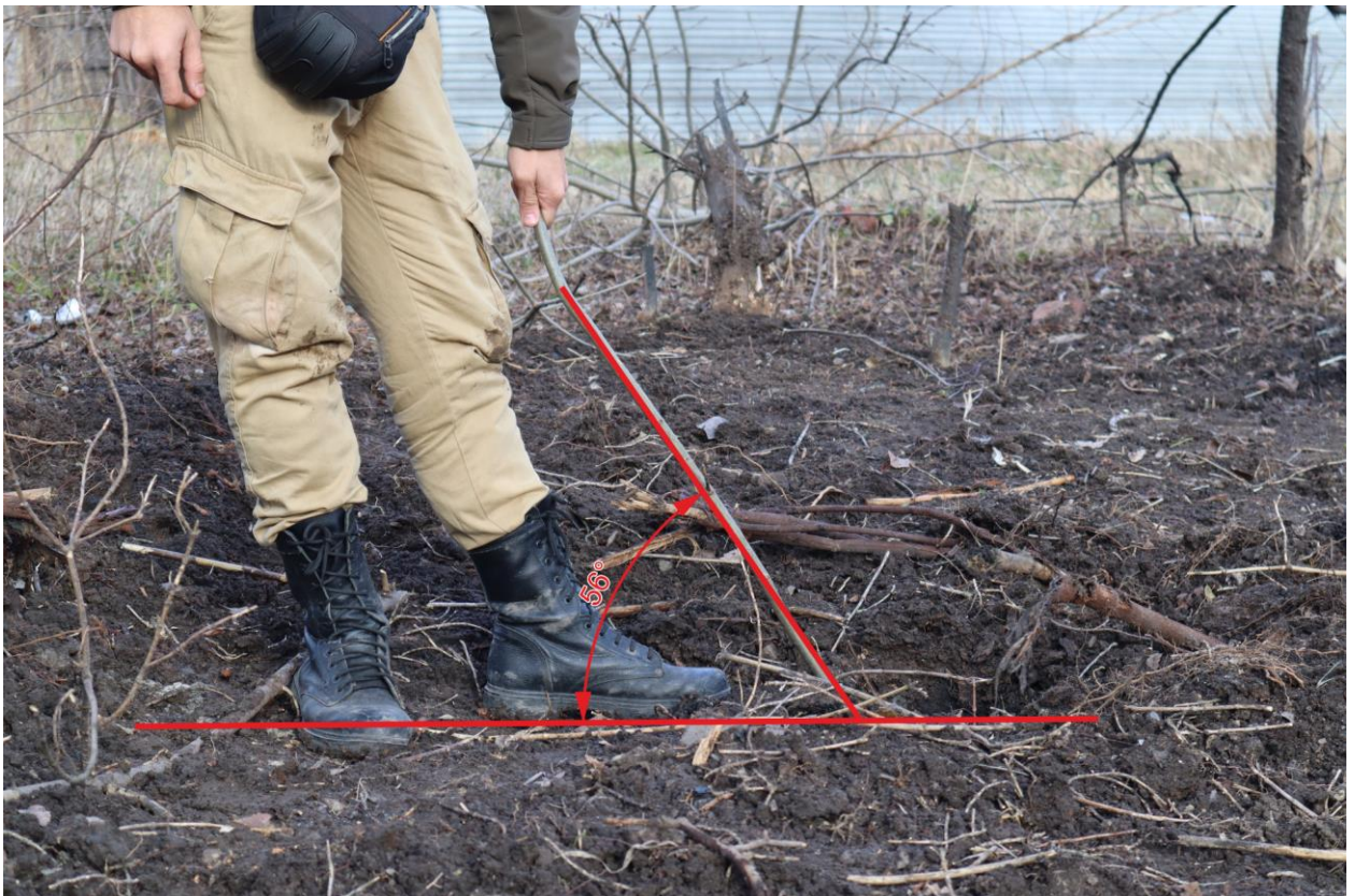
Fig. 28 – Determining the angle of impact with a horizontal surface at the site of shell hit 8
