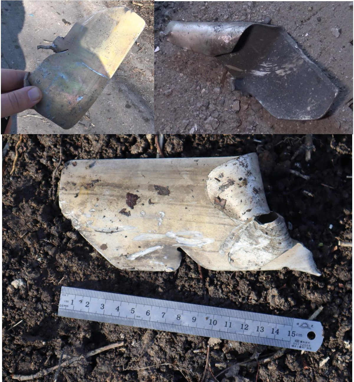
Fig. 17 - Remains of the MLRS rocket stabilizer blades discovered: top left - shell hit 5, top right - shell hit 6, bottom - shell hit 8.
