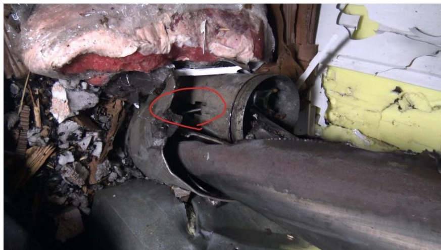
Fig. 15 - Holes at shell hit 1, characteristic of rockets of the Grad MLRS family.
