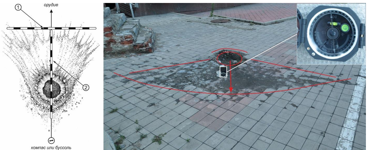
Fig. 42 – Determination of the shelling direction by the controlled fragmentation method.
