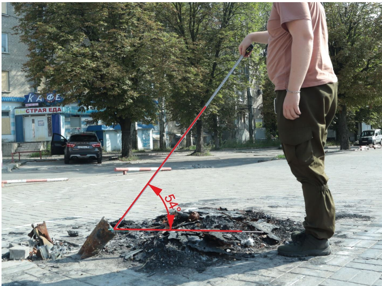
Fig. 44 – Determining the angle of impact with a horizontal surface at the site of shell hit 8 of
