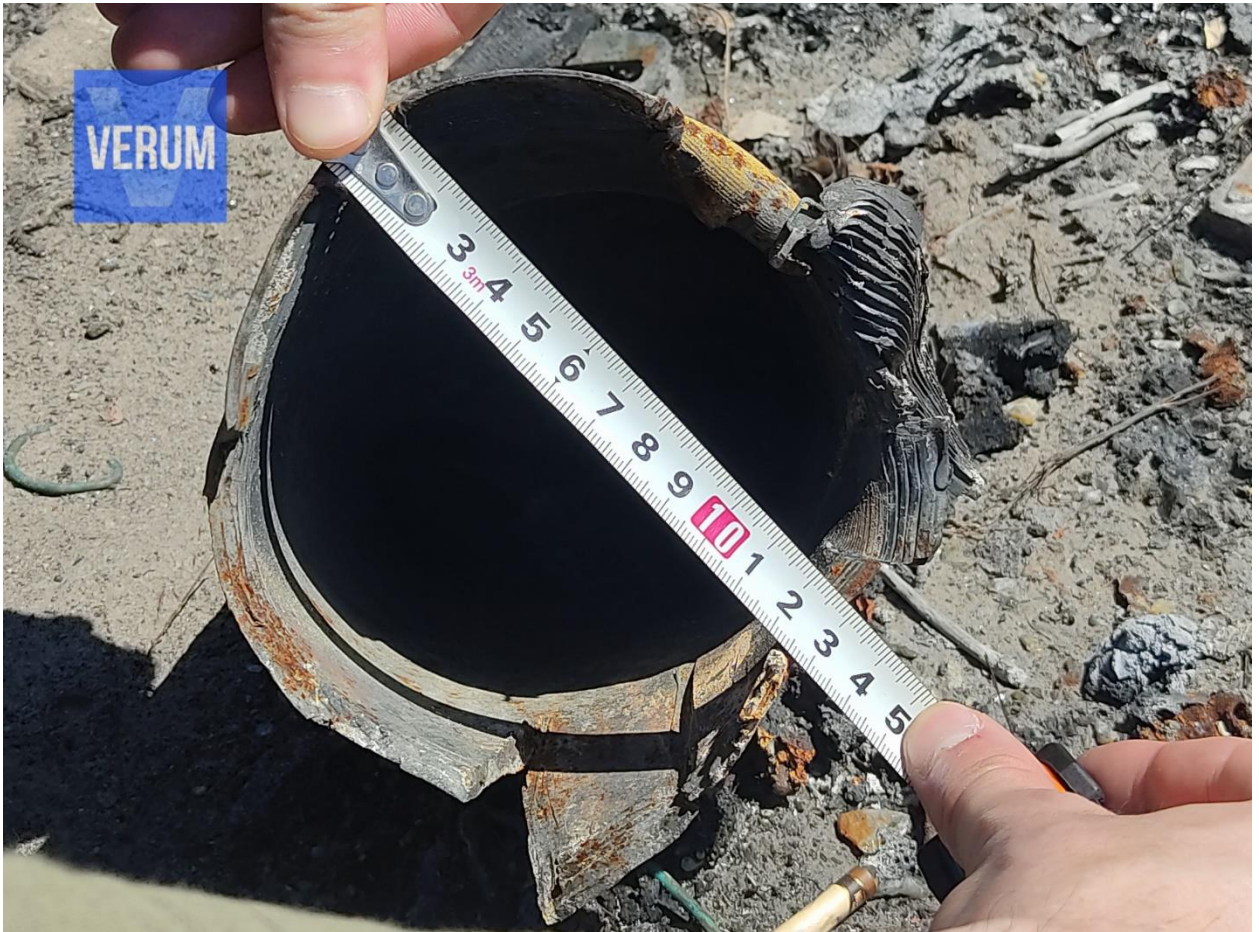
Fig. 31 – Measuring the diameter of a projectile that hit one of the cars.
