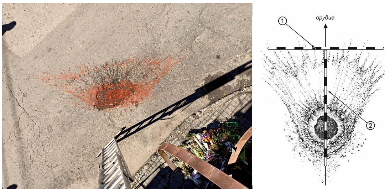
Fig. 13 – A crater at shell hit 1 and its identification by the crater type 42 .
