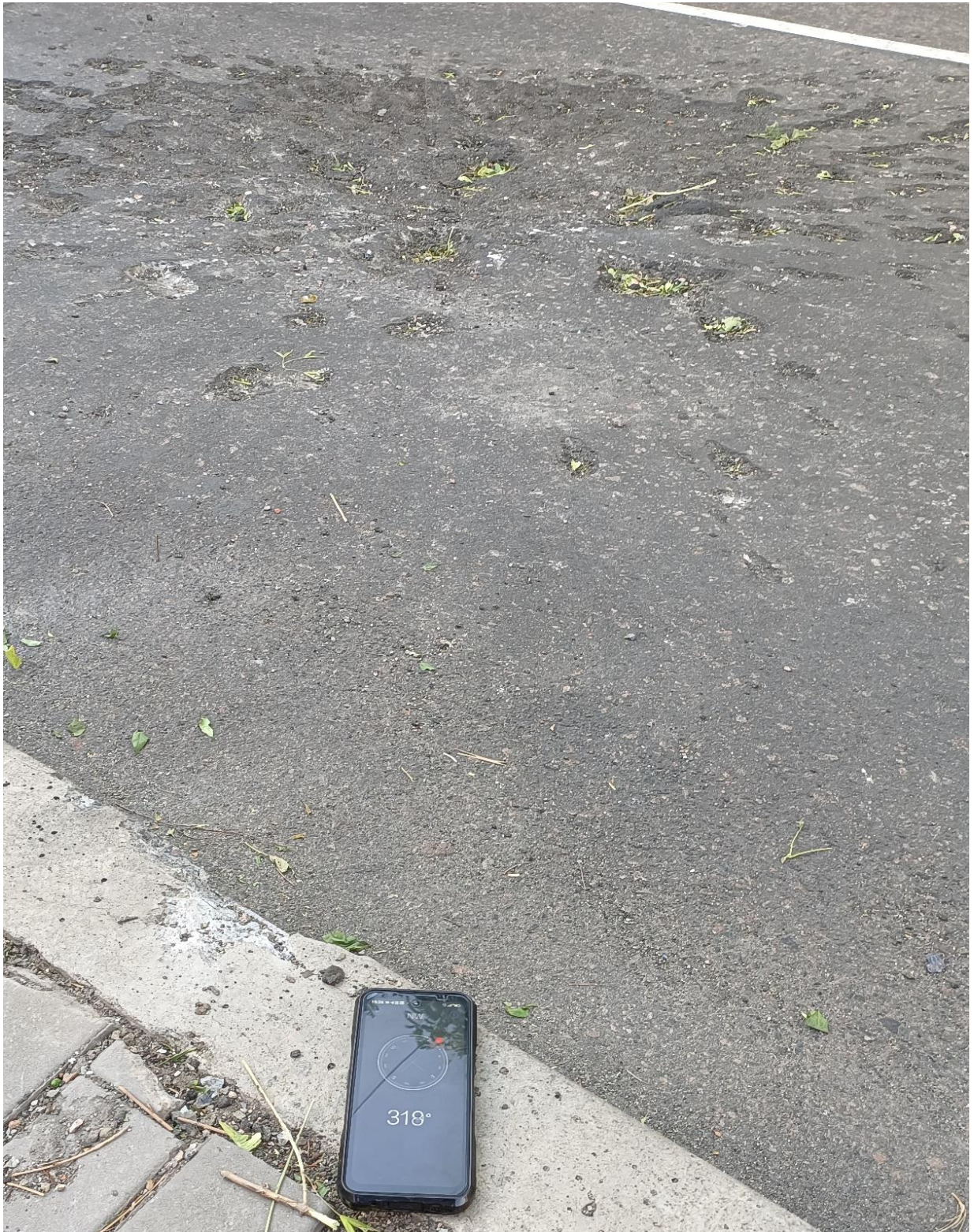
Fig. 24 – Fire direction determination in the case of shell hit 7.
