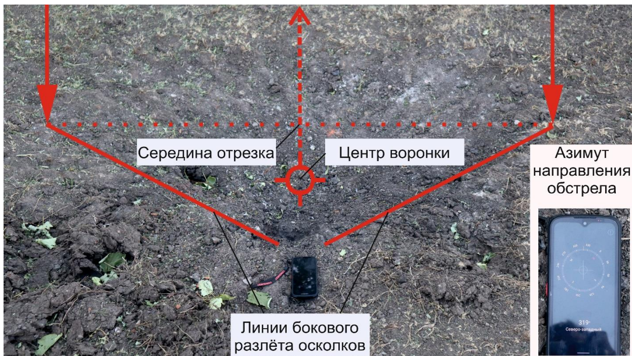
Fig. 23 - Determination of the shelling direction as exemplified by shell hit 3.
