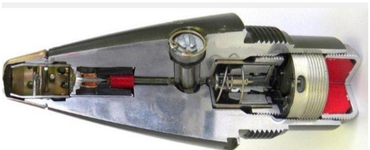
Fig. 17 – The main detonating fuze of NATO member countries for M739A1 105-mm and 155-mm ammunition 36 .
