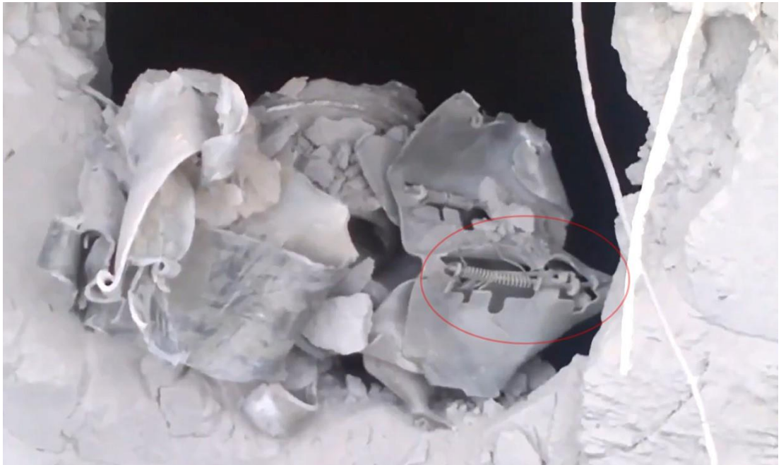
Fig. 32 - The shape of the holes for tail fin fastening which is typical for BM-21 “Grad” projectiles at the shell hit 13 42 .
