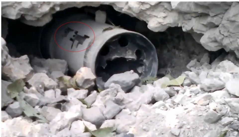
Fig. 31 – The shape of the holes for tail fin fastening which is typical for BM-21 “Grad” projectiles at the shell hit 12 41 .
