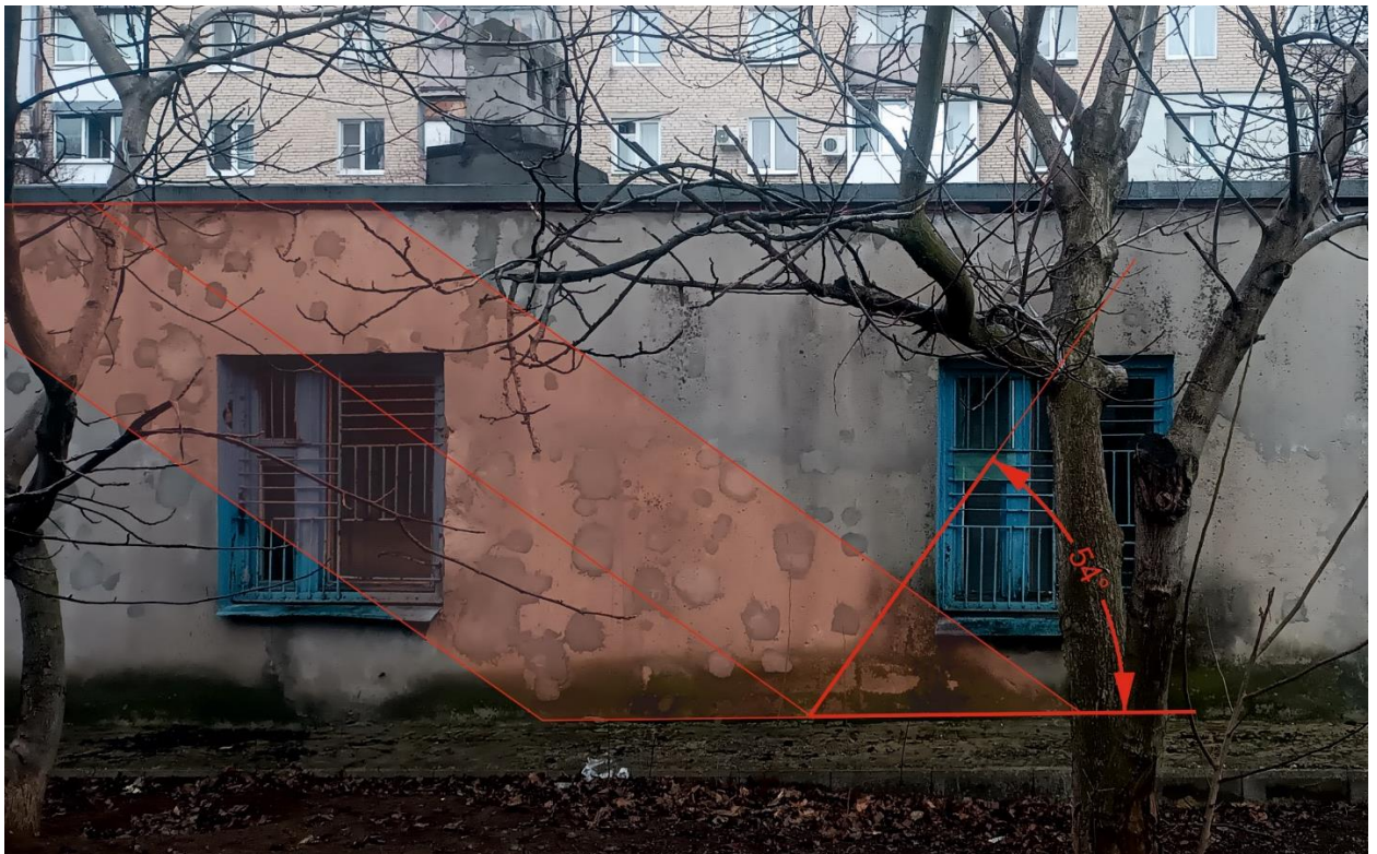
Fig. 25 – Determination of the angle of a projectile arrival based on the trace of the main scatter of fragments on the garage wall of educational complex No. 16.
