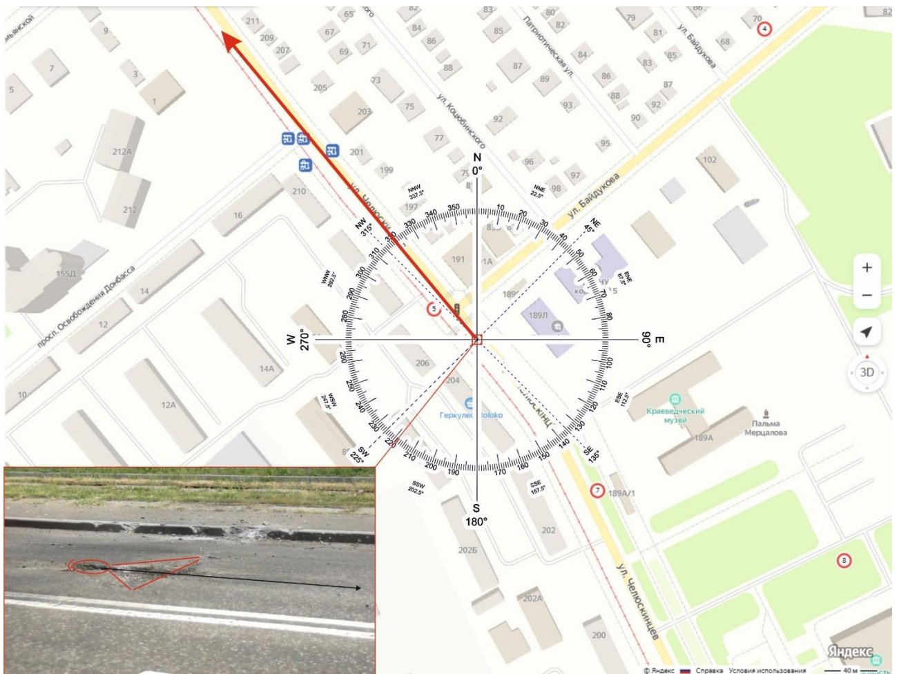
Fig. 32 – Azimuth determination at the site of shell hit 6.
