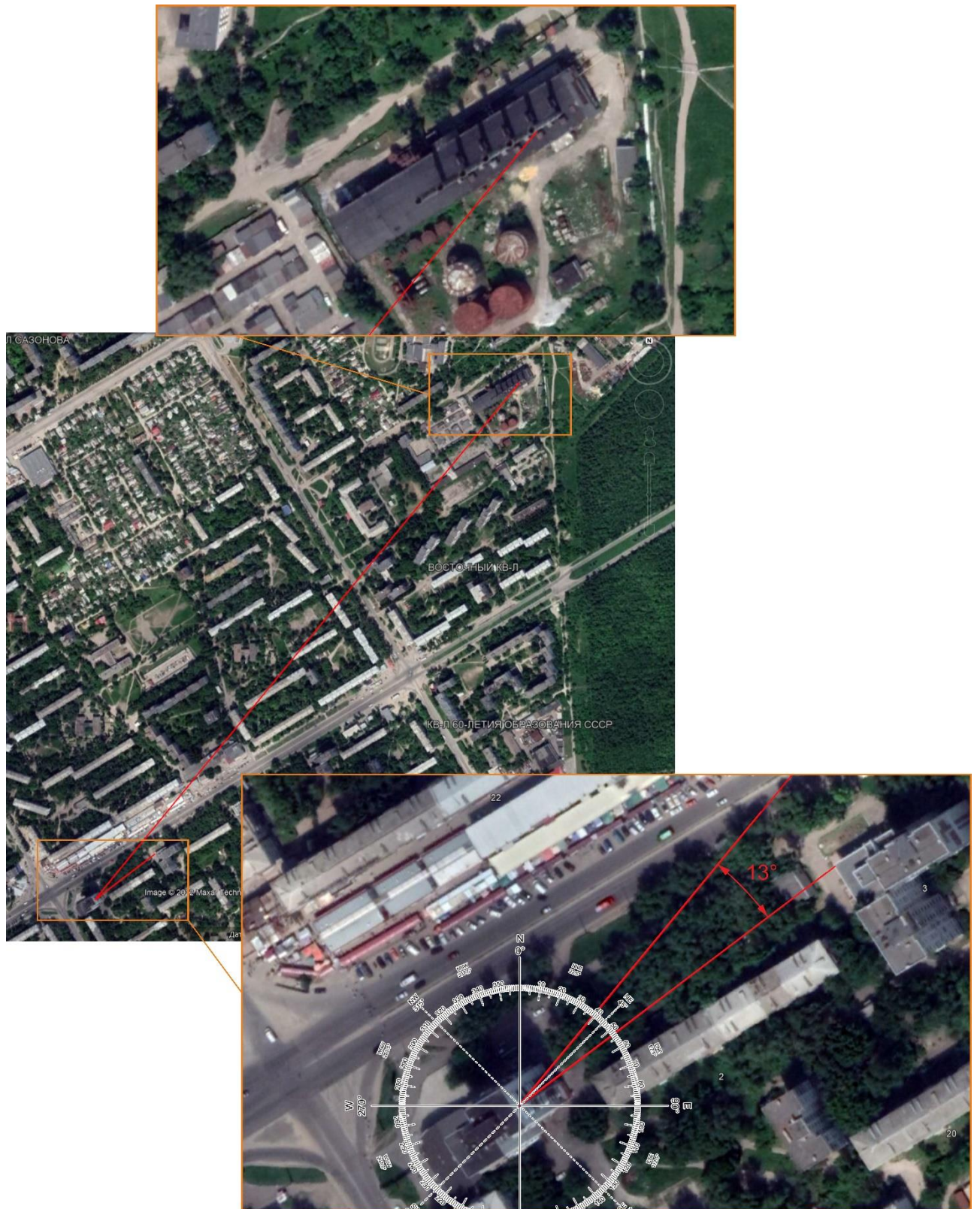
Fig. 31 – Determination of the angle between the silhouette of high-rise buildings and the pipes of the boiler facility.
